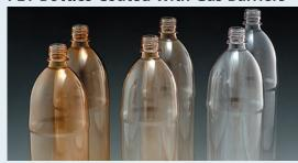
Applying gas-barrier coatings to PET bottles greatly improves gas barrier properties, which was a weak point of conventional PET bottles, and makes it possible to extend the shelf life of beverage and food products.
